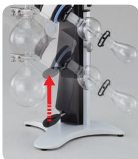
**Possible to fix jack at any elevation depending on flask's shape due to non-stepping positions**
